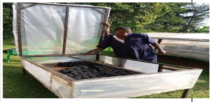
Briquettes dried in the solar dryer
