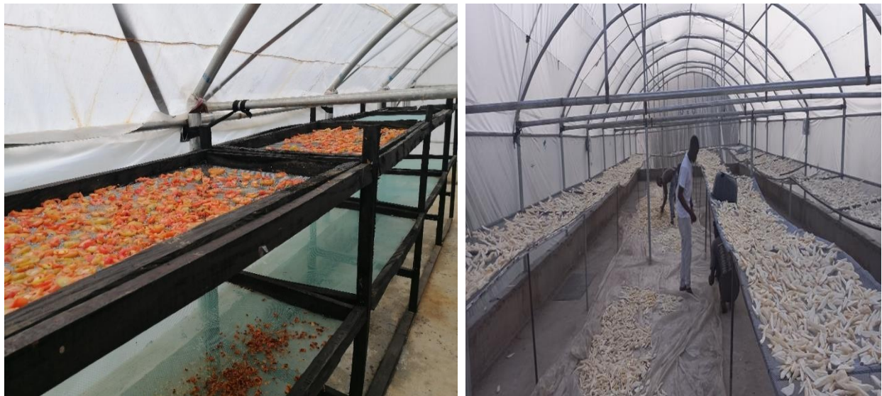
Photo: Tomato (left) and Cassava (right) loaded in the dryer during community test runs
