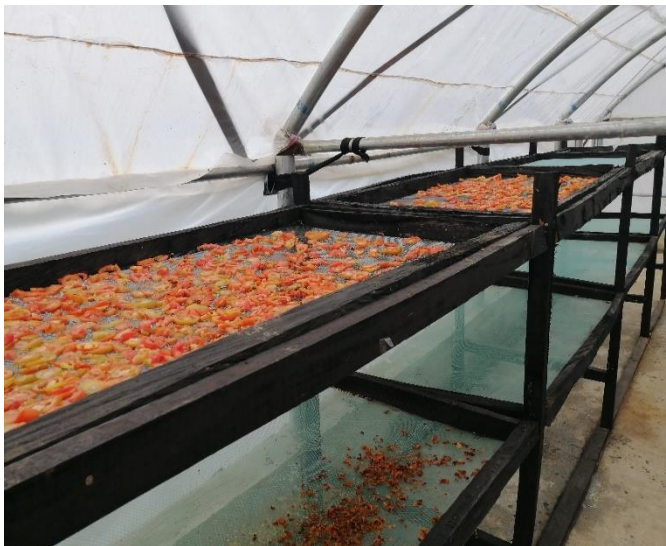
Photo: Solar dryer drying efficiency tested with tomato, a high moisture retention crop and found to be effective
