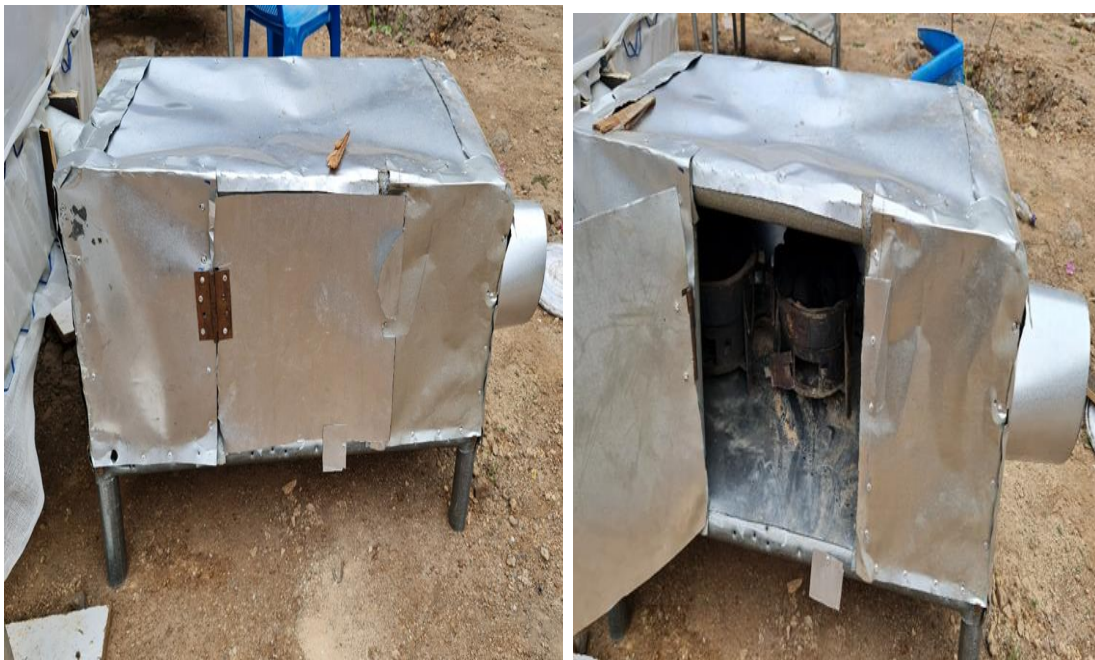
Photo: back-up heater to enhance dryer efficiency
