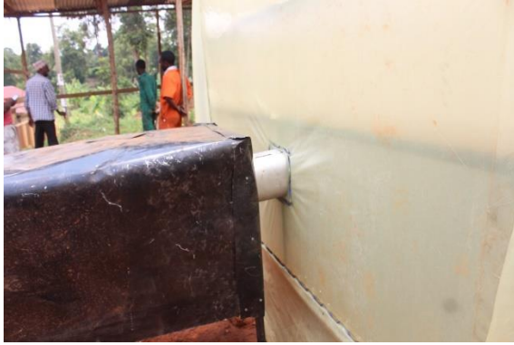
Photo left: back-up heater attached to the solar dryer; figure right: solar dryer design incorporating a back-up heater
