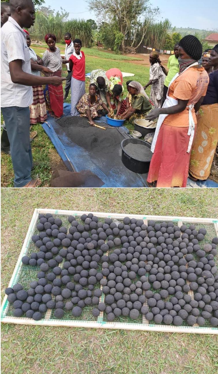
*Figure 3 Women from Nakisunga sub county trained to make briquettes and how to make raw materials using cassava waste and other agricultural waste. On the right are briquettes made by them on the first training.*
