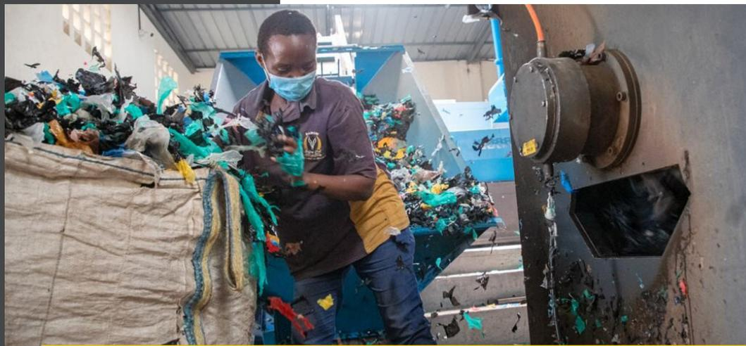
An image courtesy of Arican Development Bank (AFDB) showing a factory worker placing collected plastics in a recycling machine.
