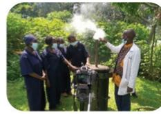
Smoke is seen in the pipe . this means waste is being carbonized
