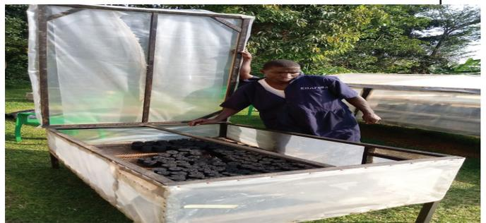
Briquettes dried in the solar dryer
