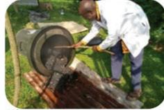
After 3-5 hours the waste carbonized turned in char ready to be crushed
