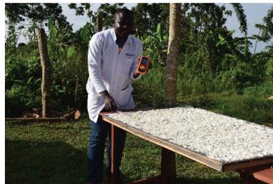
UNEP-EBAFOSA Officer hold a digital moisture meter. taking readings of samples on the raised platform / open sun drying sample
