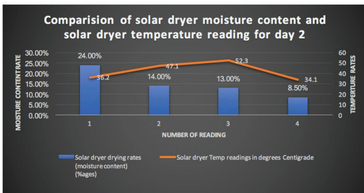
Figure 6 Comparison of solar dryer moisture content and temperature rates
