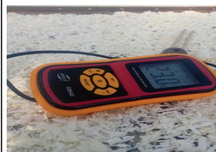
Digital Moisture meter used to measure moisture content and temperature rates of cassava chips
