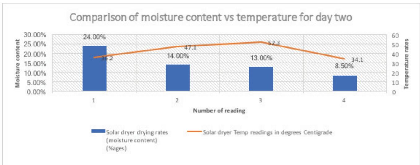
Figure 9 comparison of moisture content and temperature rates of day two readings
