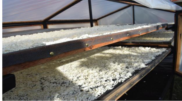
Cassava samples loaded into the solar dryer
