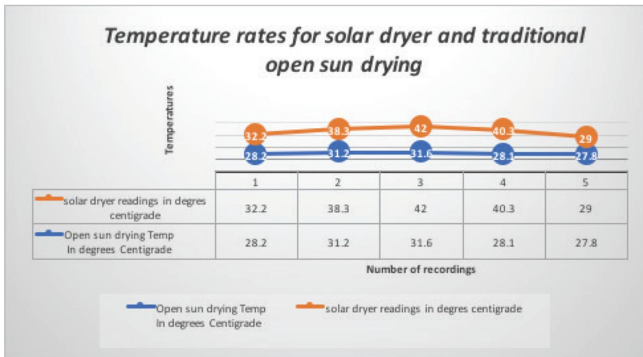
Figure 2 Temperature rates for solar dryer and traditional open sun drying day one
