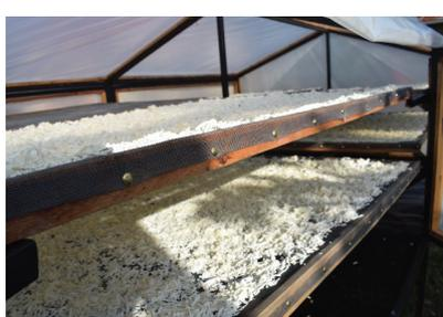
Cassava samples loaded into the solar dryer
